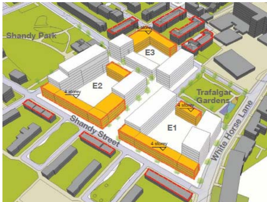
Figure 9.1 – Massing plan of Site E showing location of the lower rise elements
